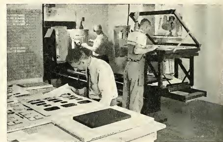
Shown here is a section of Kutztown's offset department, where the plates necessary for offset printing are produced.
