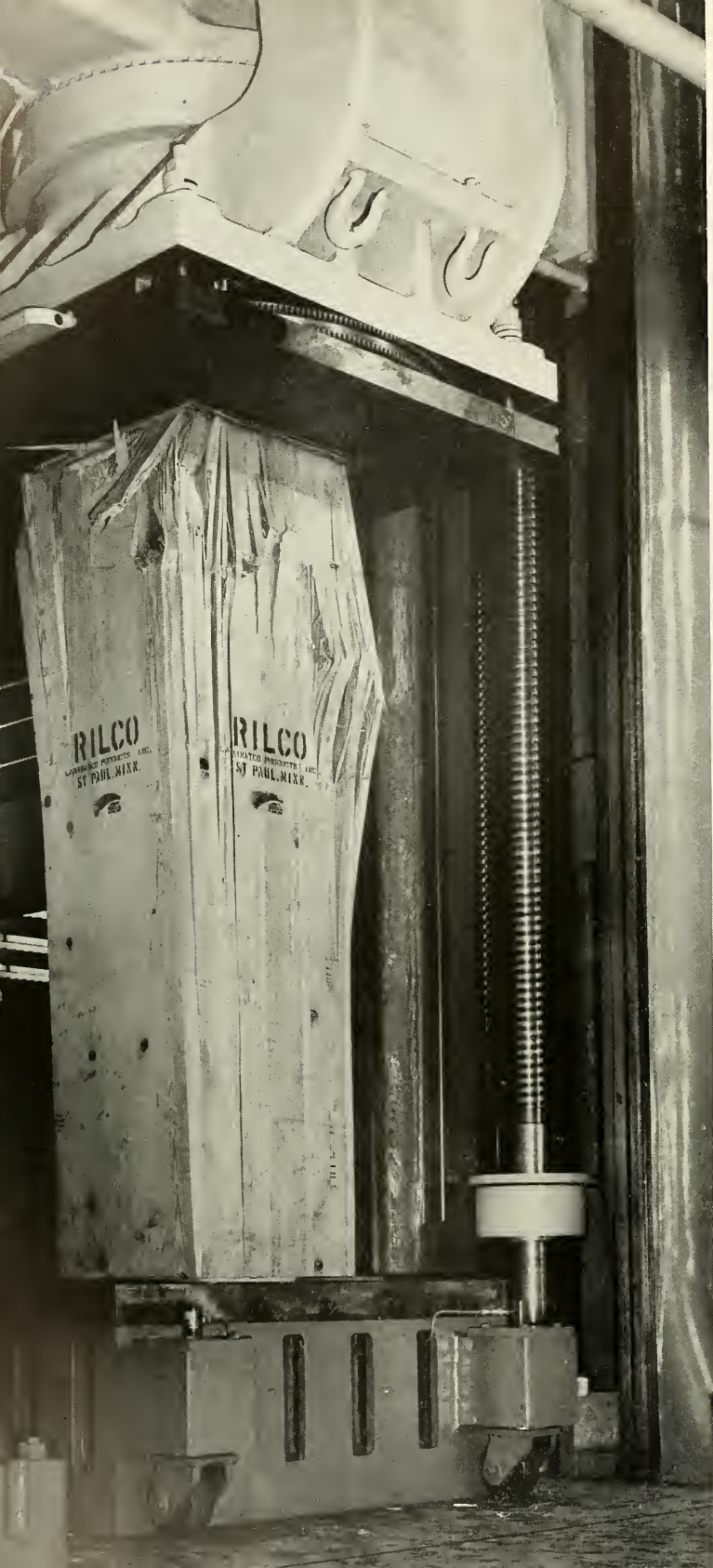
In a demonstration of the testing machine, this laminated pillar is subjected to 4,840,000 pounds of compression.
