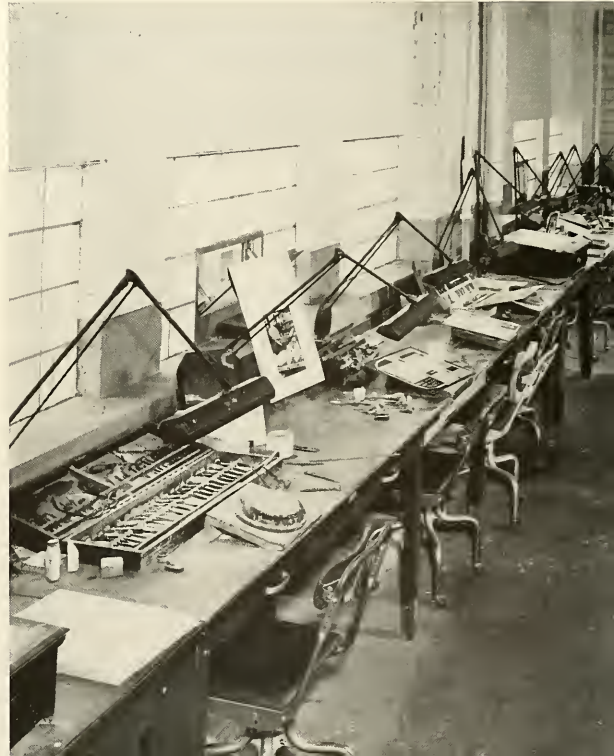
This is a section of J&O's Finishing Department where plates are checked for proper size, and any necessary tooling is done.
