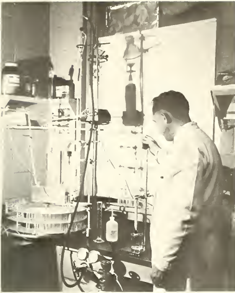
Professor J. R. Merkel separating chroma- proteins on a column with a fraction collector. These colored compounds are used to evaluate the enzyme activity of marine bacteria.
