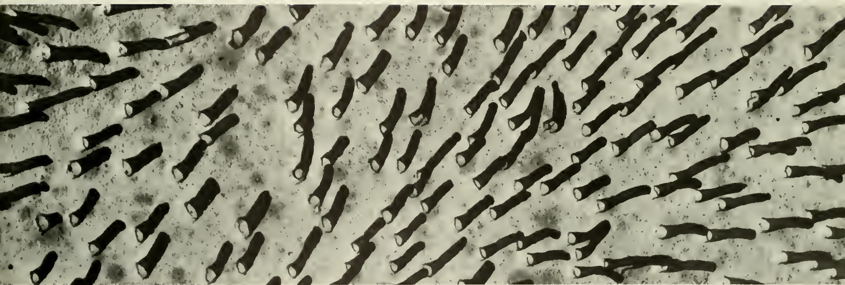
"Five o'clock shadow" is an electron micrograph showing the structure of the MnBi-Bi unidirectionally solidified eutectic. The MnBi-Bi eutectic forms long rods of MnBi, less than a micron in width, parallel to the growth direction. Magnification is 5600x.
