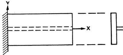
FIG. 3.35 An example of a symmetry plane containing a finite element.
