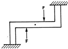
FIG. 3.31 A structure with symmetric loads.
