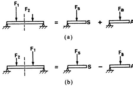
**FIG. 3.33** Superposition of symmetric and antisymmetric solutions. (a) Modeled side. (b) Unmodeled side.
