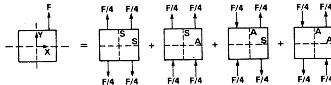
**FIG. 3.34** Multiple planes of symmetry.
