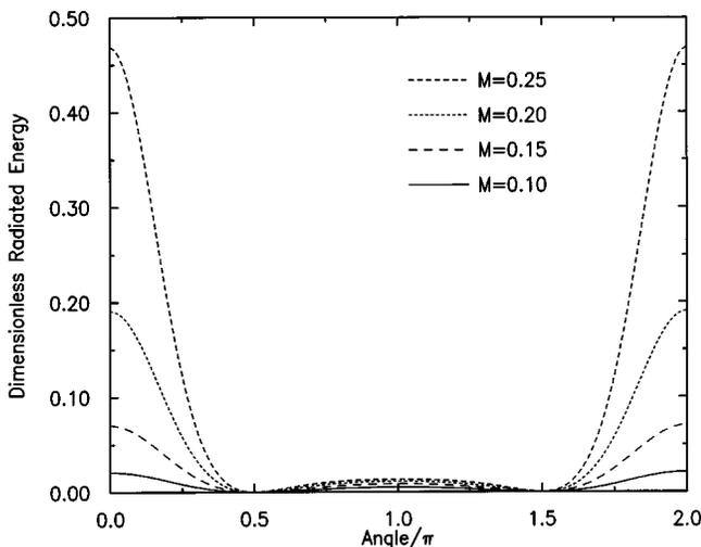
FIG. 3. Angular distribution of the instantaneously radiated energy from the moving dipole at time  $t = -\tau$ , when the dipole begins its turn-around maneuver, for Mach numbers from  $M = 0.10$  to  $M = 0.25$ .
